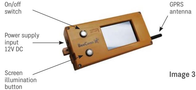
The concentrator is the basic and central unit of the device (Image 3), which periodically receives weight data from individual scales, weather station and other units.
